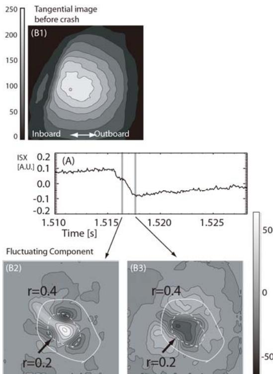
Fig.1. Line integrated tangential image of a sawtooth-like crash. Fluctuation components are shown in (B2) and (B3)
