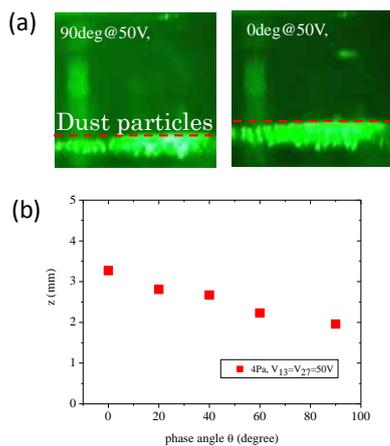
Fig.3. (a) Images of dust particles levitating in ion sheath. (b) A levitation position of dust particles as a function of phase angle  $\theta$ .
