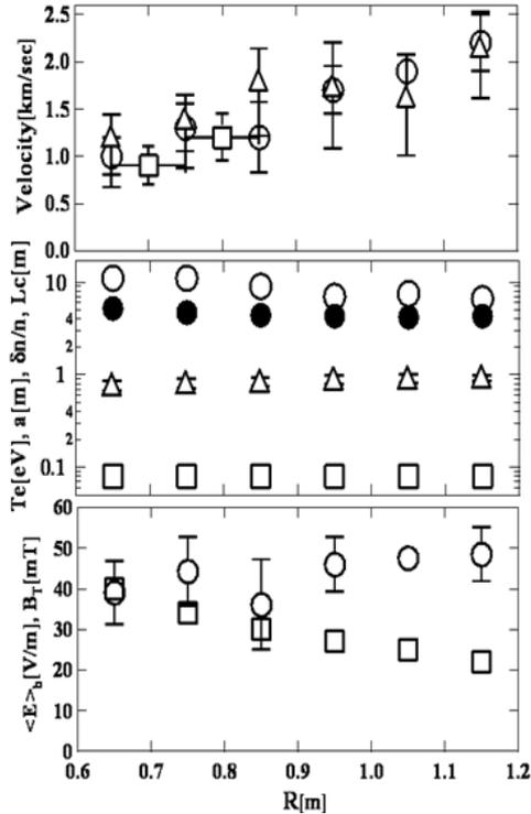
Fig. 2 Top: the radial profiles of the  $V_{E \times B}$  (circles), the  $V_{\text{image}}$ (squares) and  $V_{\text{th}}$ (triangles). Middle: Electron temperature (circles),  $\delta n/n$  (squares), blob size (triangles), and connection length (solid-circles). Bottom: the radial profiles of  $\langle E \rangle_b$  (circles) and  $B_T$  (squares). Where the  $B_z$  of  $\sim 16\text{mT}$  was applied on the mid-plane region [15].
