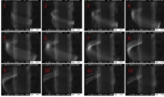
Fig. 1 Time evolution of a typical life of a blob, detach from the main plasma, radially propagate and interact with the first wall. Images were measured with the fast camera of 20000 FPS from 21.2ms to 21.75ms correspond to frame 1 – 12, shot No.:9618#.
