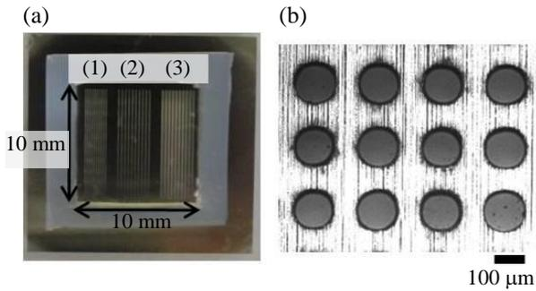
**Fig. 2.** Stainless-steel masks used in this study; (a) has three different sets of slits, (b) is the micrograph of mask which has holes.
