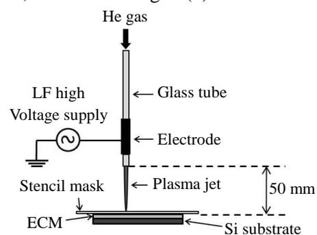
**Fig. 1.** Experimental set up for ECM patterning by LF plasma jets.
