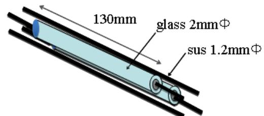
Fig. 1.(a) quadrupole of antenna system
