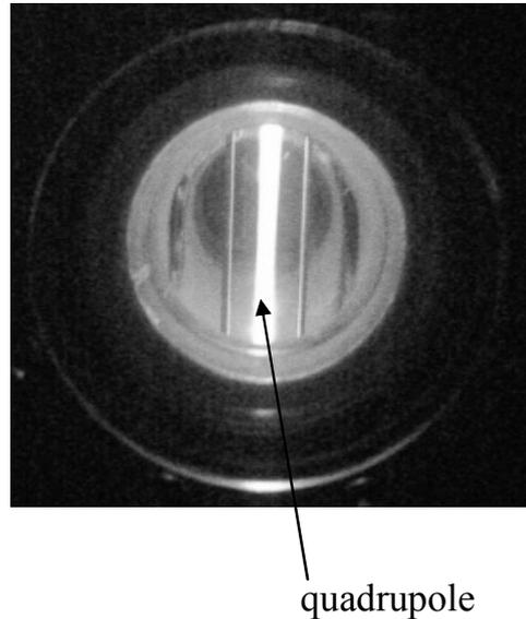
Fig. 3. An photo example of narrow RF discharge
