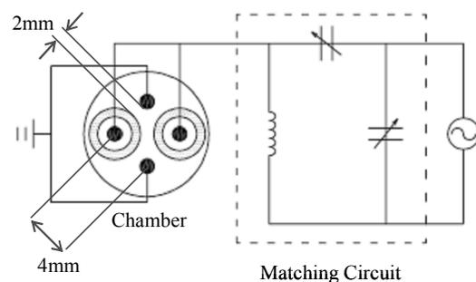
Fig. 1.(b) schematic of rf and antenna system
