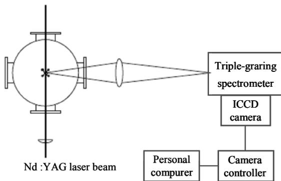
Fig. 2. An arrangement of Thompson laser scattering equipment
