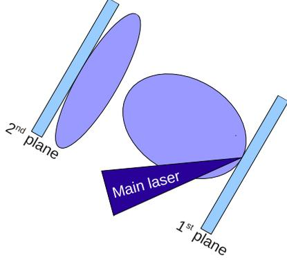
Figure 1: Schematic view of the target design. The main laser beam is focused on the 1st plane. Two planes are made of the same material.
