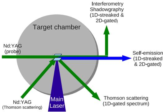
Figure 2: Experimental setup. The green line is the path of Nd:YAG laser and the blue line from target chamber center (TCC) is the path of self-emission at the wavelength of  $\sim 450$  nm.
