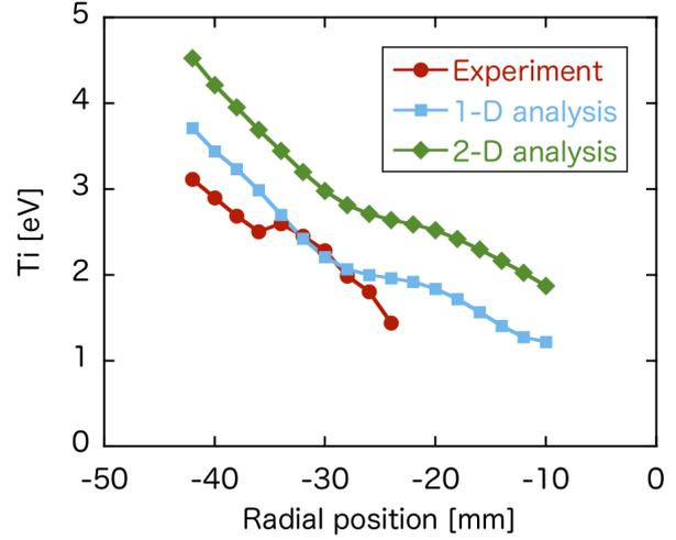
Fig.3 Comparison of  $T_i$  profile obtained by ISP measurement at the outside of the plasma column with results of analytical models of 1-D and 2-D
