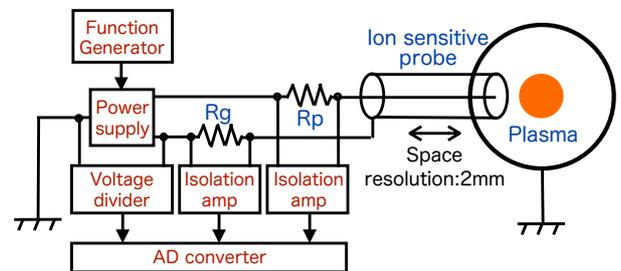
Fig.1 Schematics of ISP measurement system
