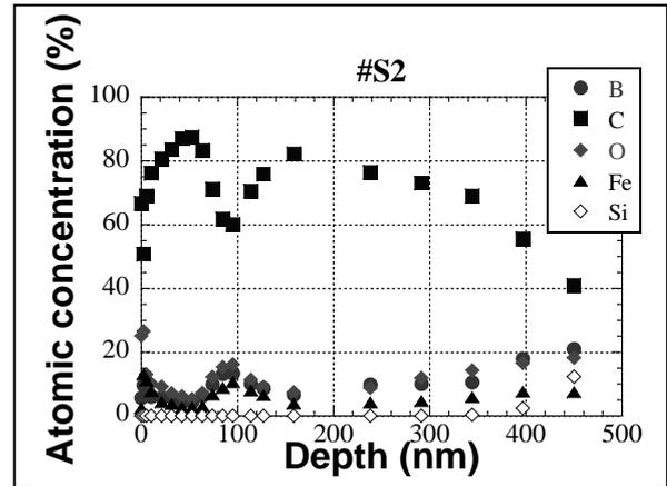
Fig.2. Atomic concentration of deposition layer on sample S2
