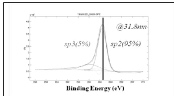
Fig.3. Fitting analysis of carbon 1s at the depth of 31.8nm on sample S2.
