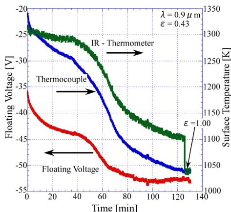
Fig.3 Cooling of Tungsten
