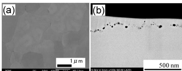
Fig.2 Recovery of W surface with nano-fiber structure. (a) : top view, (b) : cross-section view
