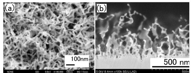
Fig.1 W surface with nano-fiber structure.
