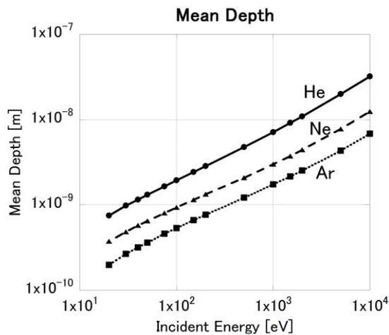
Fig. 1. Dependence of mean depth of incident particles on incident energy. Solid line with circles (●), dashed line with triangles (▲), and dotted line with squares (■) indicate the cases for helium, neon, and argon injection, respectively.
