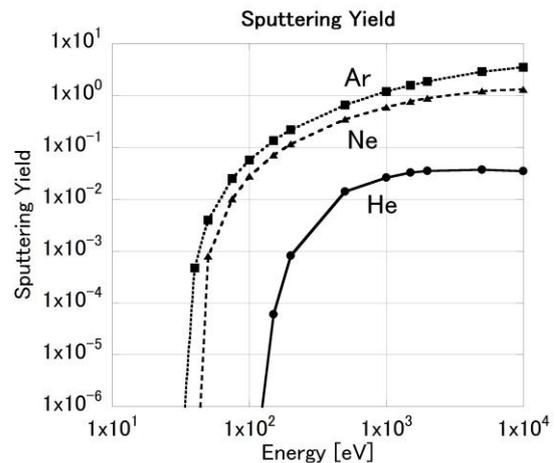
Fig. 2. Sputtering yields dependence on incident energy. Meaning of the symbols is same as Fig.1.
