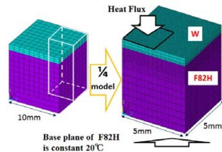
Fig.2 : 1/4 model using FEM
