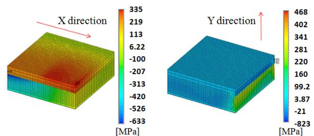
Fig.4 : X and Y direction distribution of stress
