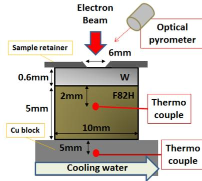
Fig.1 : Schematic illustration of the electron beam irradiation experiment
