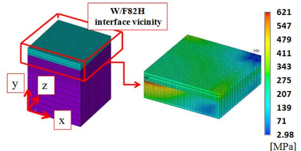
Fig.3 : Mises stress distribution at a heat flux of 8MW/m<sup>2</sup>
