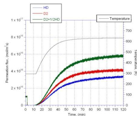
Fig. 3(b). The time evolutions of permeation fluxes of HD, D<sub>2</sub> and the sample temperature (~2h)
