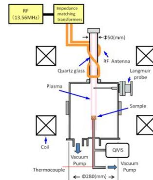
Fig. 1. Schematic diagram of the PWI simulator APSEDAS
