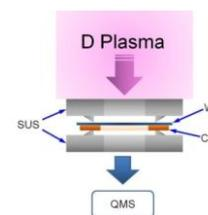
Fig. 2. Schematic diagram of the sample holder
