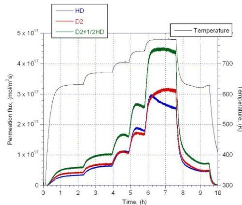
Fig. 3(a). The time evolutions of permeation fluxes of HD, D<sub>2</sub> and the sample temperature
