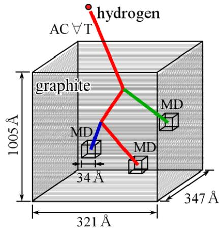
Fig.1. Schematic diagram of the BCA-MD hybrid simulation of hydrogen injection into a graphite [8].
