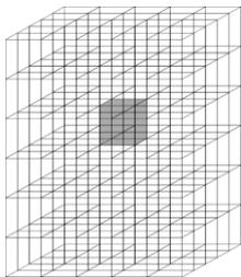
Fig.2. Amorphous material in submicrometer-scale which is divided into periodic boundary cells.
