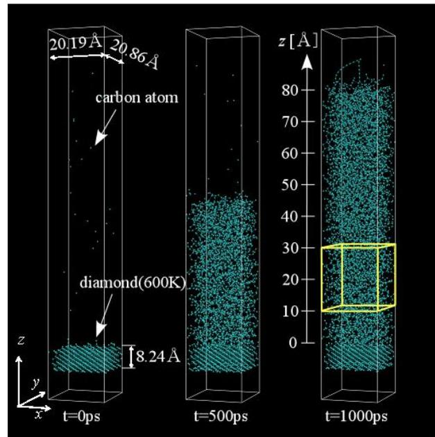
Fig.3. Simulation model for deposition [10].
