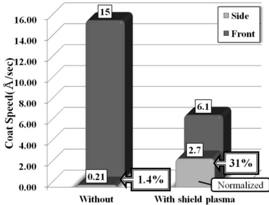
Fig.3. Results of quartz thickness monitor (Carbon)
