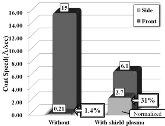
Fig.3. Results of quartz thickness monitor (Carbon)
