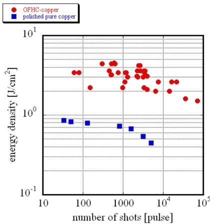
Fig. 2. Multi pulse LIDT on OFHC - copper and polished pure copper mirror.
