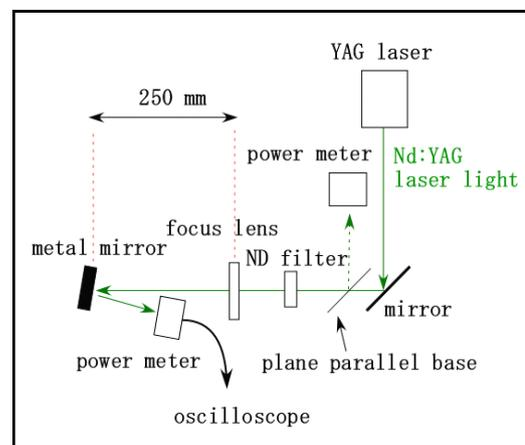
Fig. 1. Experimental measurement system
