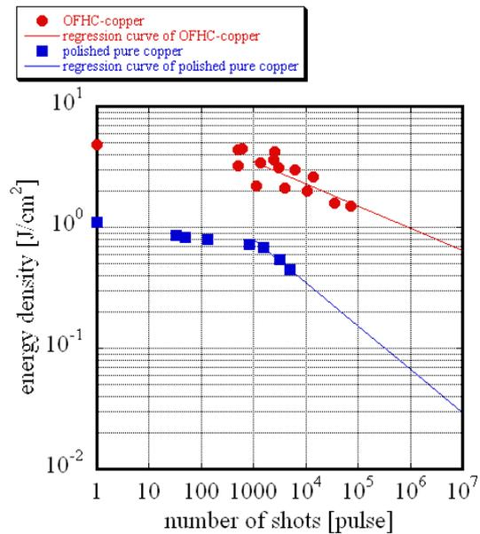
Fig. 4. Single shot LIDT, multi pulse LIDT and regression curve for more than  $10^3$  pulses on OFHC - copper and polished pure copper mirror.
