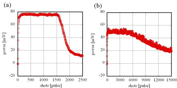
Fig. 3. For polished pure copper, energy density is  $6.8 \times 10^{-1} \text{ J/cm}^2$  for (a),  $4.5 \times 10^{-1} \text{ J/cm}^2$  for (b).
