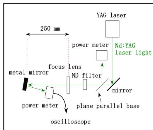
Fig. 1. Experimental measurement system
