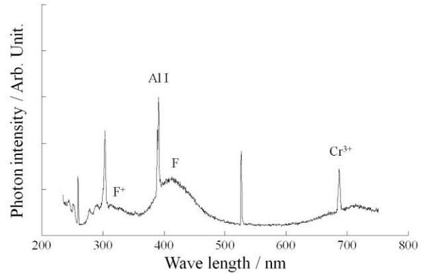
Fig.2 luminescence spectrum induced by 266 nm Nd:YAG laser irradiation
