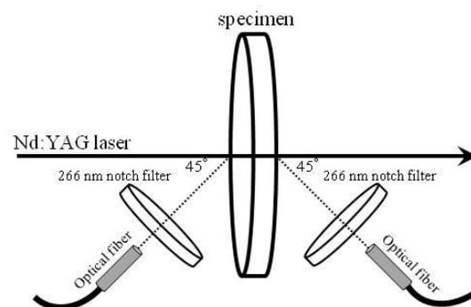
Fig. 1 schematic diagram of experimental arrangement
