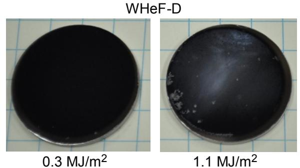
Fig. 4 Photographs of W samples with pulsed D plasma loads.
