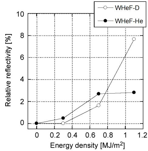
Fig. 3 Relative reflectivity of fuzzy W surfaces after pulsed plasma bombardment.
