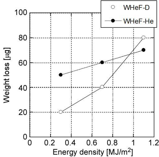
Fig. 1 Weight loss of fuzzy W samples exposed to D and He pulsed plasma loads.
