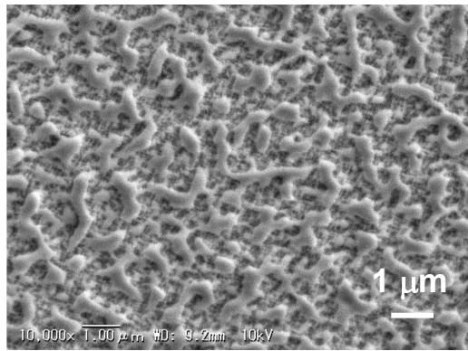
Fig. 2 SEM image of a W surface with 10 pulsed He plasma shots at  $Q \sim 0.3 \text{ MJ/m}^2$ .
