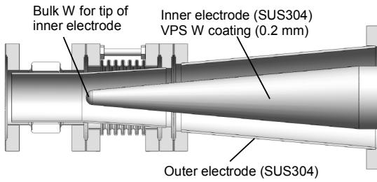
Fig. 2 Inner and outer electrodes in the MCPG device.
