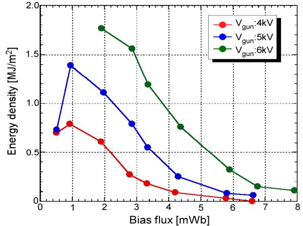
Fig. 3 Dependences of the energy density of the pulsed plasma on the bias flux.
