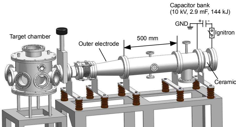
Fig. 1 Magnetized coaxial plasma gun device
