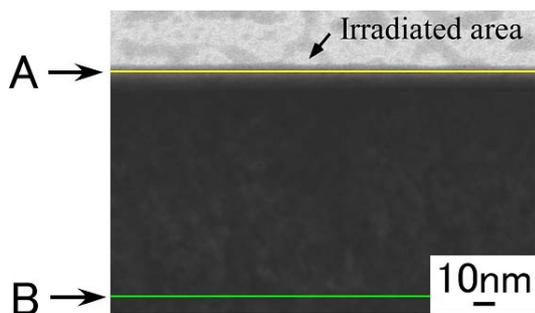
**Figure 2.** Cross-sectional SEM micrograph of W target that was exposed at exposed to pure Ar plasma.
