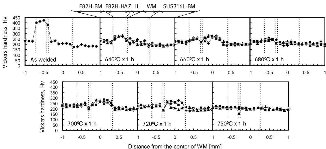
Fig. 1. Cross-sectional Vickers hardness distribution in the as-welded and post-welding heat treated F82H/SUS316L EBW joints (PWHT temperatures: 640, 660, 680, 700, 720, 750°C)
