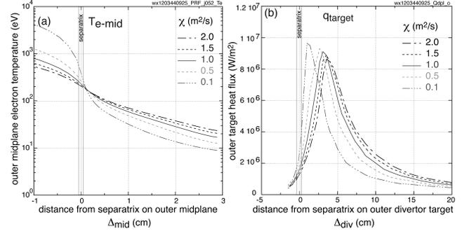
Fig.3. Dependence on the thermal diffusivity  $\chi$  of (a) electron temperature profile on the outer midplane  $T_{e\text{-mid}}$  and (b)  $q_{\text{target}}$ .
