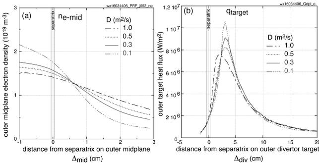
Fig.2. Dependence on the particle diffusivity  $D$  of (a)  $n_{e\text{-mid}}$  and (b)  $q_{\text{target}}$ .
