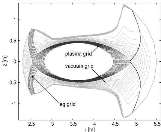
Fig. 3: Generated grid in the plane  $\phi=162$ .
