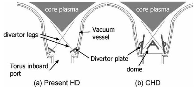
Fig. 4: (a) Open and (b) closed divertor configuration in the cross section.
