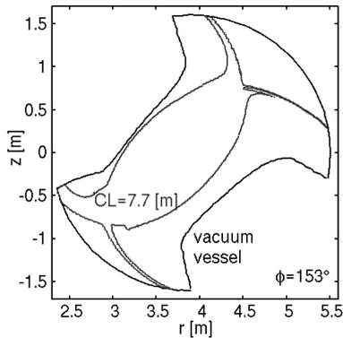
Fig. 1: Contour of connection length for 7.7m where the toroidal angle  $\phi$  is 153 degree.
