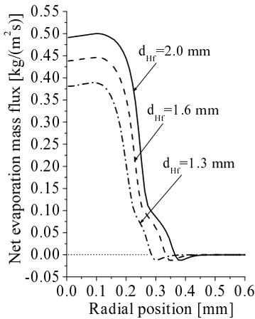
Fig. 4: Radial distribution of net evaporated mass flux from Hf cathode for different cathode diameters
