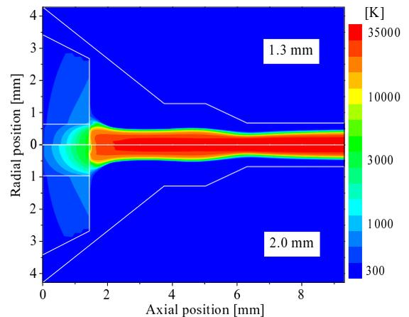
Fig. 2: Temperature distribution of arc plasma with cathode diameter of 1.3 mm and 2.0 mm
