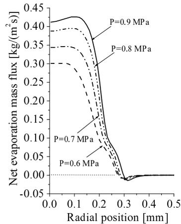
Fig. 6: Radial distribution of net evaporated mass flux from Hf cathode for different gas pressures
