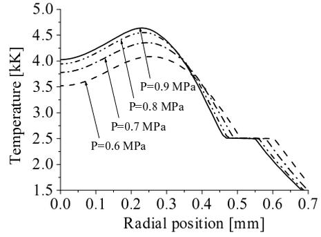
Fig. 5: Radial distribution of surface temperature of Hf cathode for different gas pressures
