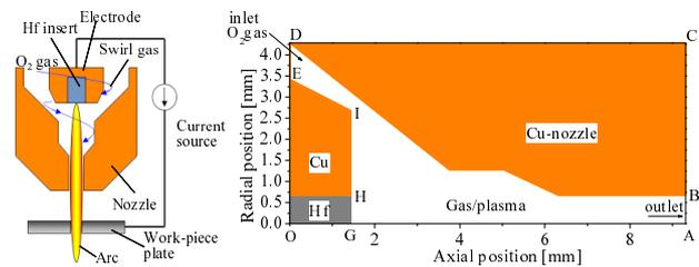
Fig. 1: Arc model and calculation space
