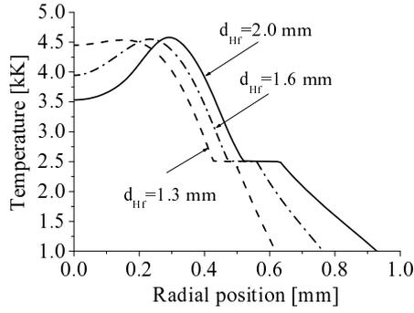
Fig. 3: Radial distribution of surface temperature of Hf cathode for different cathode diameters
