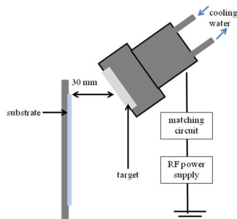
Fig. 1. Schematic diagram experimental setup.
