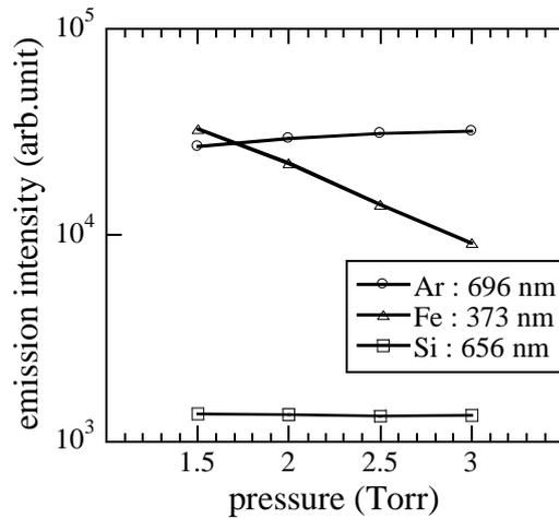
Fig. 2. Pressure dependence of the emission intensities of Ar, Fe, and Si.
