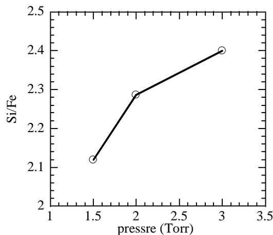
Fig. 3. Dependence of Si/Fe composition ratio on pressure.
