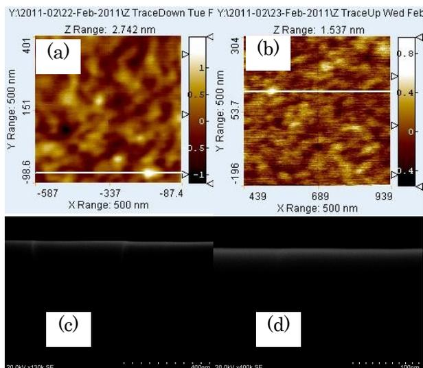
Fig.3. (a) AFM and (c,d) SEM image of HfO<sub>2</sub> film by PAALD on SiO<sub>2</sub>/Si(100) with pure O<sub>2</sub> ICP. (b) Use of O<sub>2</sub>(1%)/Ar(99%) ICP reduces surface roughness.
