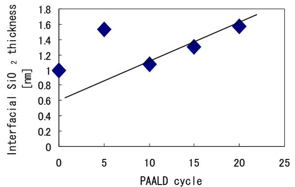
Fig. 4. Interfacial SiO<sub>2</sub> layer thickness with the PAALD cycle.
