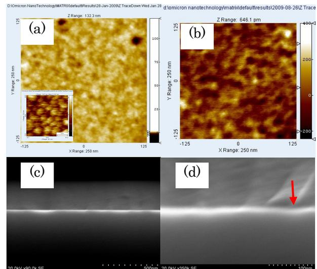
Fig.1. (a) AFM and (c,d) SEM image of  $\text{HfSiON}$  film by PEPVD with  $\text{N}_2$  ICP exposure to Hf metal (2.5nm) on  $\text{SiO}_2/\text{Si}(100)$ . (b)  $\text{Hf}_{0.9}\text{Ti}_{0.1}\text{SiON}$  film grown by PEPVD.
