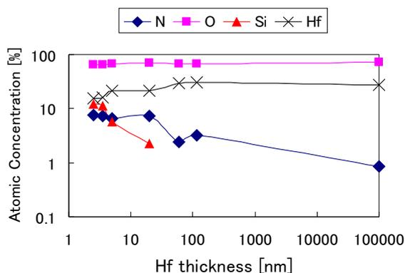
Fig.2. Atomic concentration change of HfSiON film grown by PEPVD for increased initial Hf thickness.
