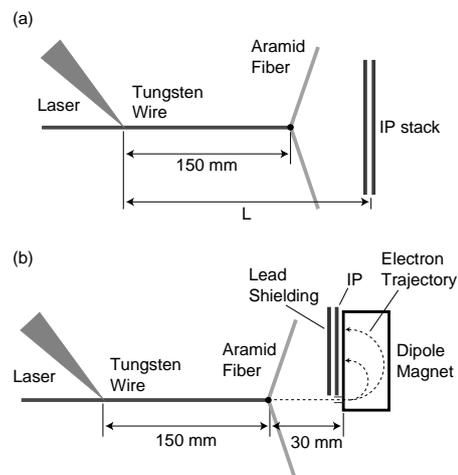
Fig.1 (a) Experimental setup to observe emitted electrons using stacked IPs. (b) Experimental setup to observe the energy distribution of electron beam along the wire and through a 0.5-mm aperture.
