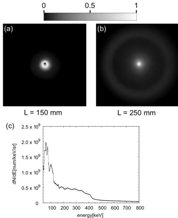
Fig.2 (a) and (b) Typical single-shot images of electron emission obtained on the second layer IP with  $L = 150$  mm,  $L = 250$  mm, respectively. The color scale is set independently for images for maximum contrast. The actual dimension of the images are  $35\text{ mm} \times 35\text{ mm}$ . Center black spot seen in (a) is a hole with diameter of 1 mm is made in the IP. (c) Typical energy distribution of electrons.
