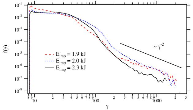
Figure 2: Energy distribution functions of the electrons in logarithmic scales.
