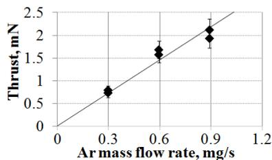
Fig. 2. Thrust as a function of the Ar gas mass flow rate.
