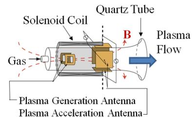
Fig. 1 Concept of Lissajous Method
