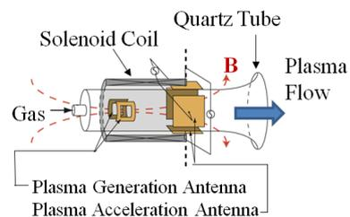
Fig. 1 Concept of Lissajous Method
