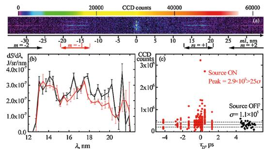
Fig.1 (a) Raw CCD image. (b) Spectra in the diffraction order of  $m=1$  and  $m=-1$ . (c) CCD counts within the 1<sup>st</sup> diffraction order.
