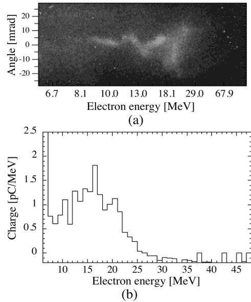
Fig.2 (a) Typical image of an electron beam in energy space and (b) a projection of the image onto the energy axis at  $n_e=4.4 \times 10^{19}$  cm<sup>-3</sup>.
