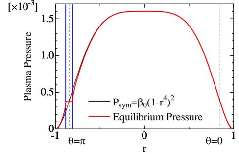
Figure1: Equilibrium pressure profiles in the cases with methods of (a) diffusion equation and (b) tracing field line. Blue lines denote the position of the separatrix of the magnetic island. The dotted lines show the positions of the rational surface.
