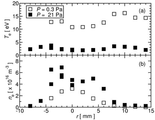
Fig.3. Radial profiles of the electron temperature(a) and density(b) with (closed squares) and without (open squares) gas puffing obtained at the test region.
