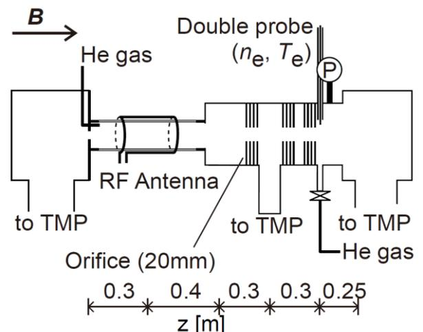
Fig. 1. A schematic of the DT-ALPHA device.
