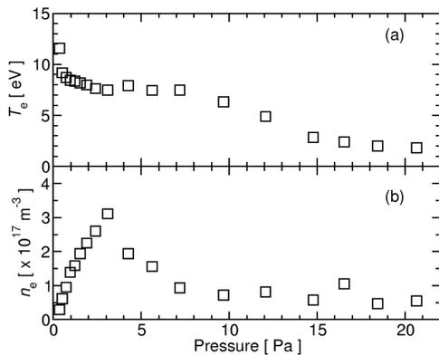
Fig.2. Neutral pressure dependence of the electron temperature(a) and density(b) obtained at the test region,  $r = 0 \text{ mm}$ .
