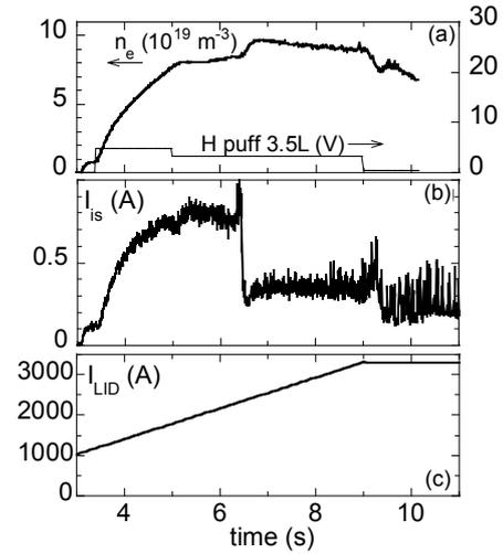
Fig. 3. Time traces of (a) line averaged density and gas puff wave form, (b) the divertor particle flux, (c) RMP coil current.
