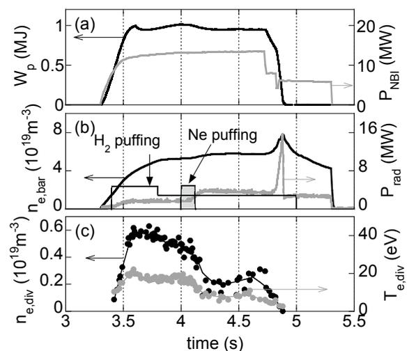
Fig. 1. Typical time evolutions of (a) plasma stored energy ( $W_p$ ) and NBI power ( $P_{\text{NBI}}$ ), (b) line averaged density ( $n_{e,\text{bar}}$ ), radiation power ( $P_{\text{rad}}$ ) and gas-puffing, (c) electron density ( $n_{e,\text{div}}$ ) and temperature ( $T_{e,\text{div}}$ ) in the divertor (torus inboard-side).
