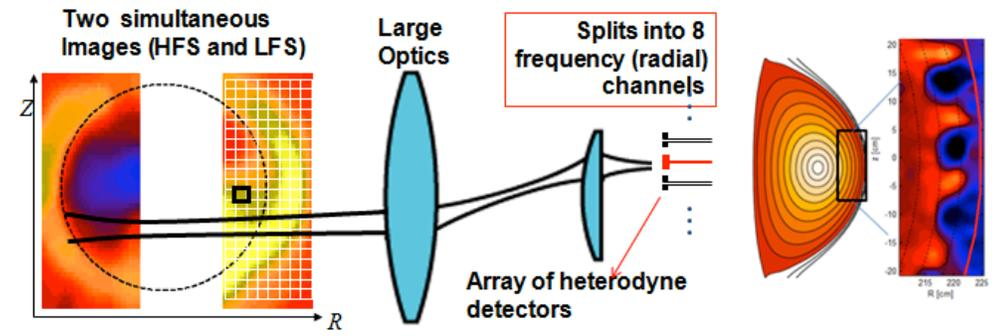
Fig.1. Schematic of the ECEI system (simultaneous measurement of two images at high and low field sides) and the structure of ELMs at the edge of the KSTAR plasma is shown.
