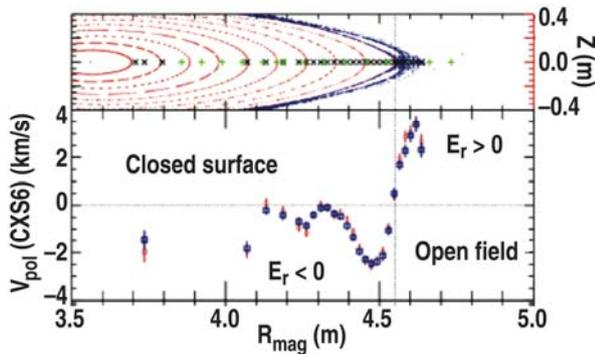
Fig. 2. (a) Closed flux surfaces bounded by a stochastic magnetic field region on the horizontal midplane where CXSS measurements are made (x's and +s), (b)  $v_{pol}$  profile from CXSS measurements showing a sharp reversal from negative flows in the closed surface region to positive in the open field region.
