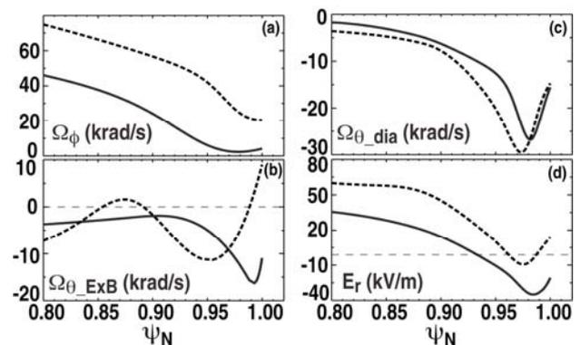
Fig.1. Change in the (a) toroidal ( $\Omega_\phi$ ), (b) poloidal ExB ( $\Omega_{\theta\_ExB}$ ), (c) poloidal diamagnetic ( $\Omega_{\theta\_dia}$ ) rotation and (d) radial electric field ( $E_r$ ) with (dashed) and without (solid) the RMP in DIII-D shot 123306.
