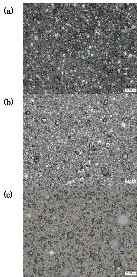
Fig. 2 Aerosol particles generated by colliding ablation plumes for (a) Li-Pb, (b) Pb-Pb and (c) Li-Li target combinations on Pyrex glass substrates.
