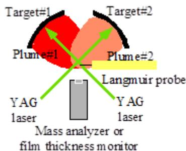
Fig. 1 A schematic diagram of the LEAF-CAP setup [4].
