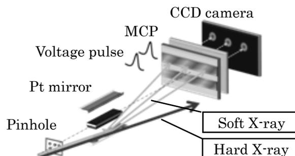
Figure 1 The schematic diagram of XFC
