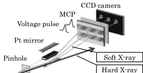
Figure 1 The schematic diagram of XFC
