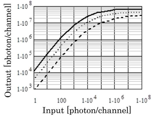
Figure 3 Input vs. Output gain curves of the MCP, at 900V (solid), 800V (dotted) and 700V (dashed)
