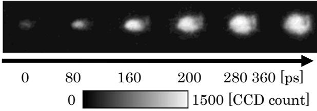
Figure 2 X-ray images of imploded core plasma (#34140)
