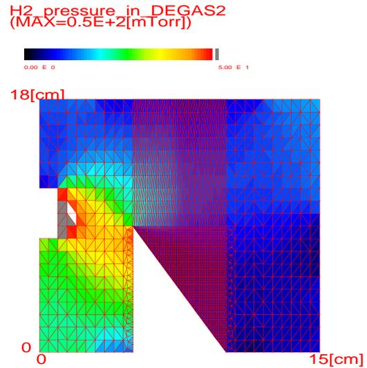
Fig.4: Hydrogen molecular pressure result with the old inclined target mesh model.
