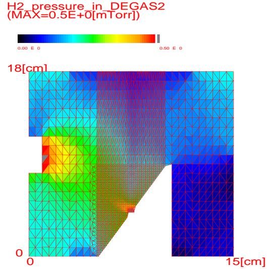
Fig.3: Hydrogen molecular pressure result with the old inclined target mesh model.
