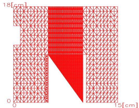
Fig.2: Simulation mesh model for V-shaped target, which was improved from those used for Fig.3 in [3].
