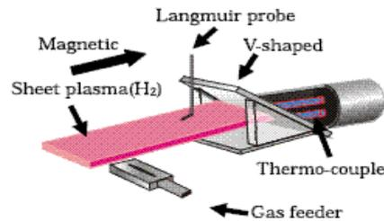
Fig.1: Schematic drawing of V-shaped target plate of TPDSheet-IV.
