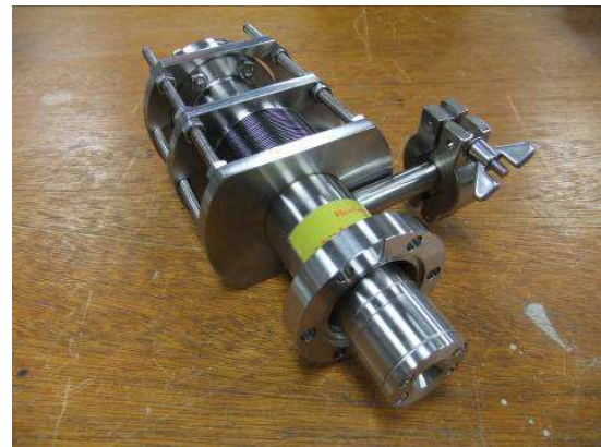
Fig.1: A soft-X ray array detector using AXUV photo-diode array and aluminum thin foil.
