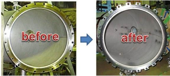
Fig.2. Photos of poloidal sections of the poloidal flanges before and after modification
