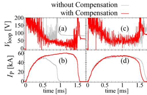
Fig.4. Time evolution of loop voltage  $V_{\text{loop}}$  and plasma current  $I_p$  with and without the compensation coils before ( (a), (b) ) and after ( (c), (d) ) modification
