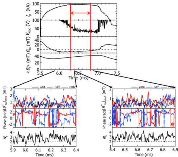
Fig.2: A 100kA discharge in RELAX with MHD behavior.
