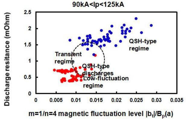
Fig.3: Discharge resistance vs.  $m=1/n=4$  magnetic fluctuation level.
