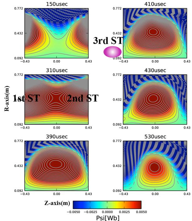
Fig. 3 R-Z poloidal flux contours when two ST merges together and the 3<sup>rd</sup> ST merge with the produced main ST.
