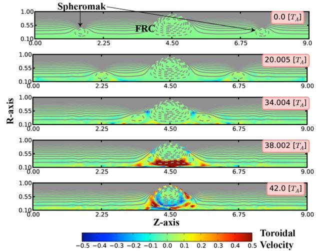
Fig.2 R-Z contours of poloidal flux and toroidal velocity (in color) when two small spheromak merge with the center main FRC (the MHD simulation).
