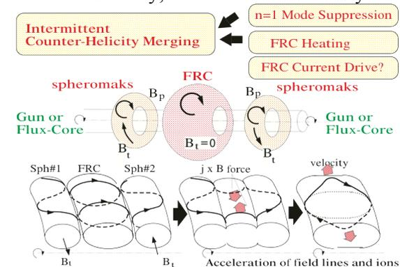
Fig.1. Continuous generation of sheared flow by multiple merging for stability / heating FRC.[]
