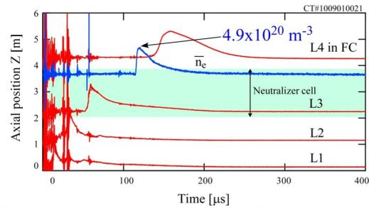
Fig. 2. Typical evolution of PIN diode signals and the CT density along CT's path.
