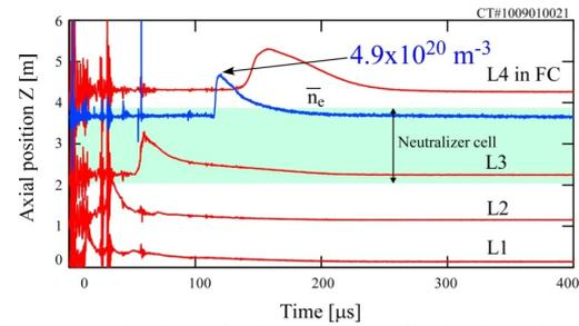
Fig. 2. Typical evolution of PIN diode signals and the CT density along CT's path.
