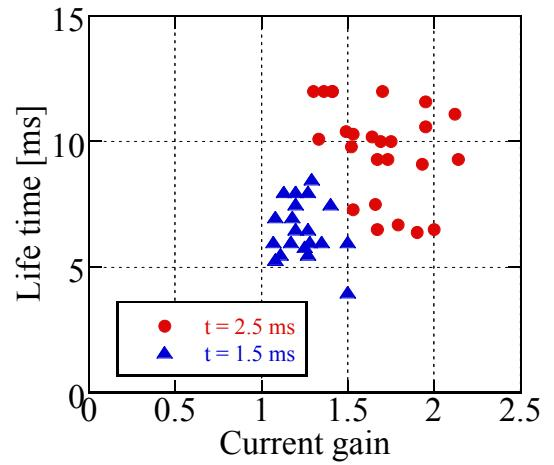
Fig.3. Comparison of the current gain and the life time between the second pulse timing at  $t \sim 2.5$  ms and  $t \sim 1.5$  ms
