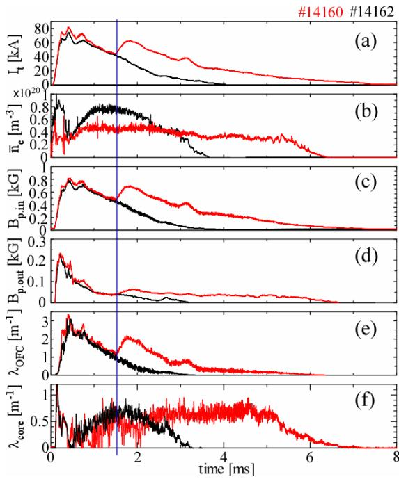
Fig.2. Time evolution of (a)  $I_t$ , (b)  $\langle n_e \rangle$ , (c)  $B_{\text{p,in}}$ , (d)  $B_{\text{p,out}}$ , (e)  $\lambda_{\text{OFC}}$ , (f)  $\lambda_{\text{core}}$ , in the comparison of single (#14162) and double pulsed discharges (#14160)
