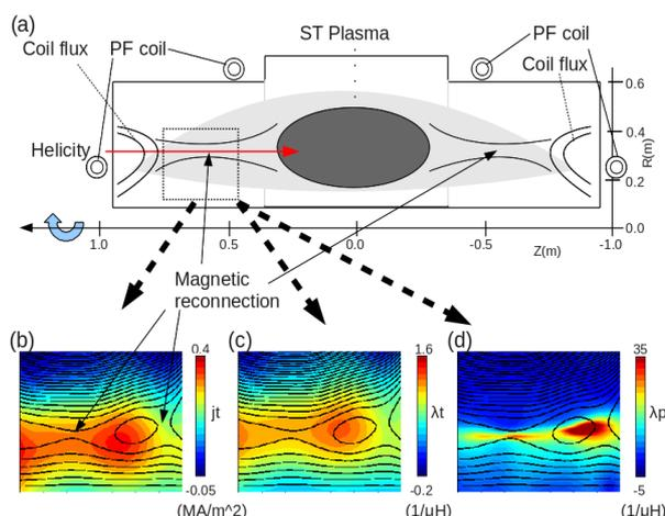
Fig1. (a) Experimental setup of UTST device with two pairs of PF coils on each side. Color contours of the measured 2-D poloidal magnetic flux with (b) toroidal current density  $jt$  (c) toroidal eigen-values  $\lambda t$  and (d) poloidal eigen-values  $\lambda p$
