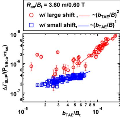
Fig.1. Fast ion loss flux dependence on fluctuation amplitude of TAE measured with magnetic probe.
