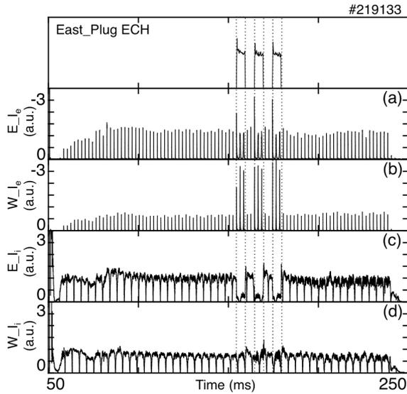
Fig.2. Temporal evolution of end loss electron current at the (a) east end, (b) west end, and end loss ion current at the (c) east end, (d) west end. The P-ECH power of about 200 kW is applied from  $t = 150$  ms to 180 ms with 100%, 100 Hz square wave power modulation.
