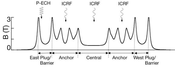
Fig.1. Axial magnetic field intensity and locations of heating systems for P-ECH modulation experiment.
