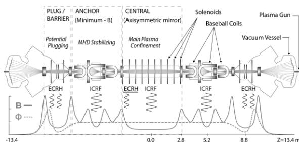
Fig.1. The schematic view of the GAMMA 10
