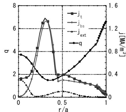
Fig.2. Profiles of safety factor  $q$ , total current density  $j_t$ , bootstrap current density  $j_{bs}$  and external current density  $j_{ext}$ .
