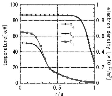
Fig.1. Profiles of electron temperature  $T_e$ , ion temperature  $T_i$  and electron density  $n_e$ .
