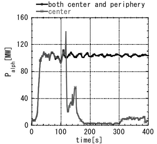
Fig.3. Time evolution of alpha heating power in both cases.
