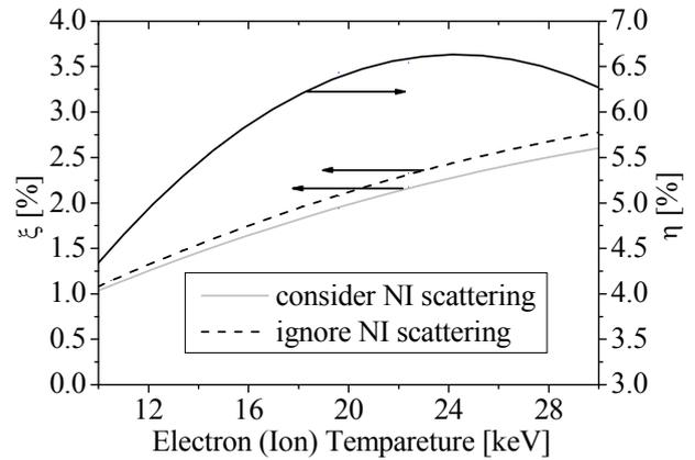
Fig.3 Temperature dependence of rate of energy loss and decreasing rate of energy loss by NI scattering
