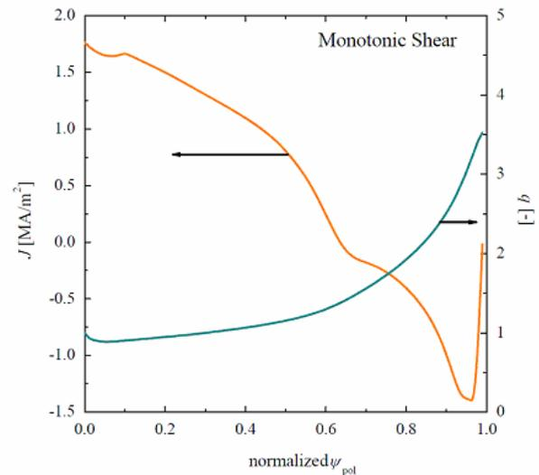
Fig.1. Safety factor and current distribution assumed this calculation [7]
