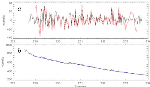
Fig.2. 0.5ms STWAS result: *a*. extracted fluctuation with 2kHz high pass FFT filter (red) and STWAS (black); *b*. raw signal (black) and "background" by STWAS (blue)
