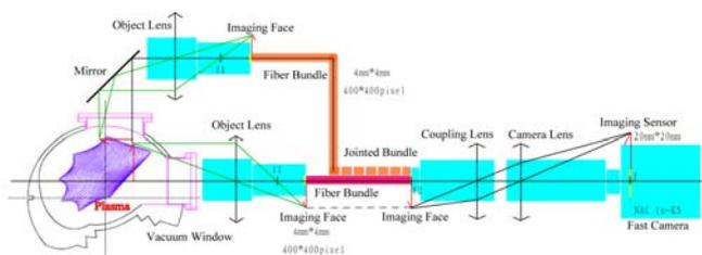
Fig.1. #11.5 Fast Camera System on Heliotron J
