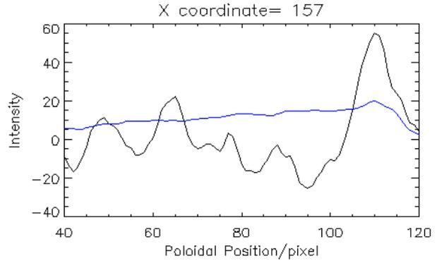
Fig.4. Fluctuation signal along a poloidal direction line at specified time point (black) and standard deviation during studied period (blue)
